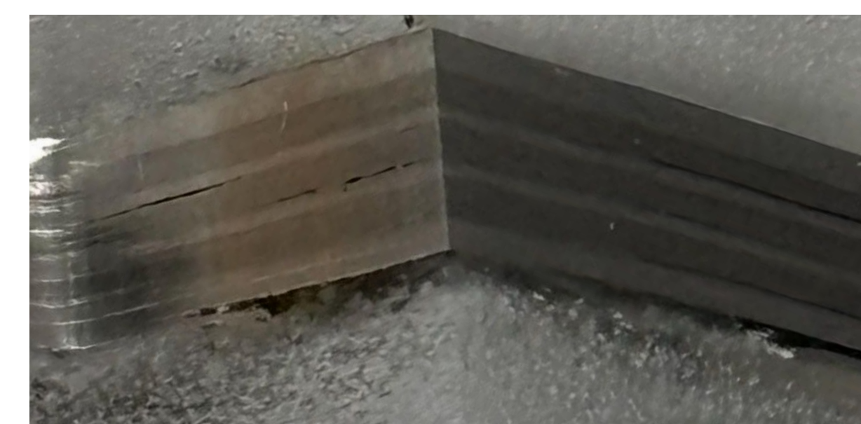
Polished cross section showing intermetallic (dark grey) and metallic (grey) layers
