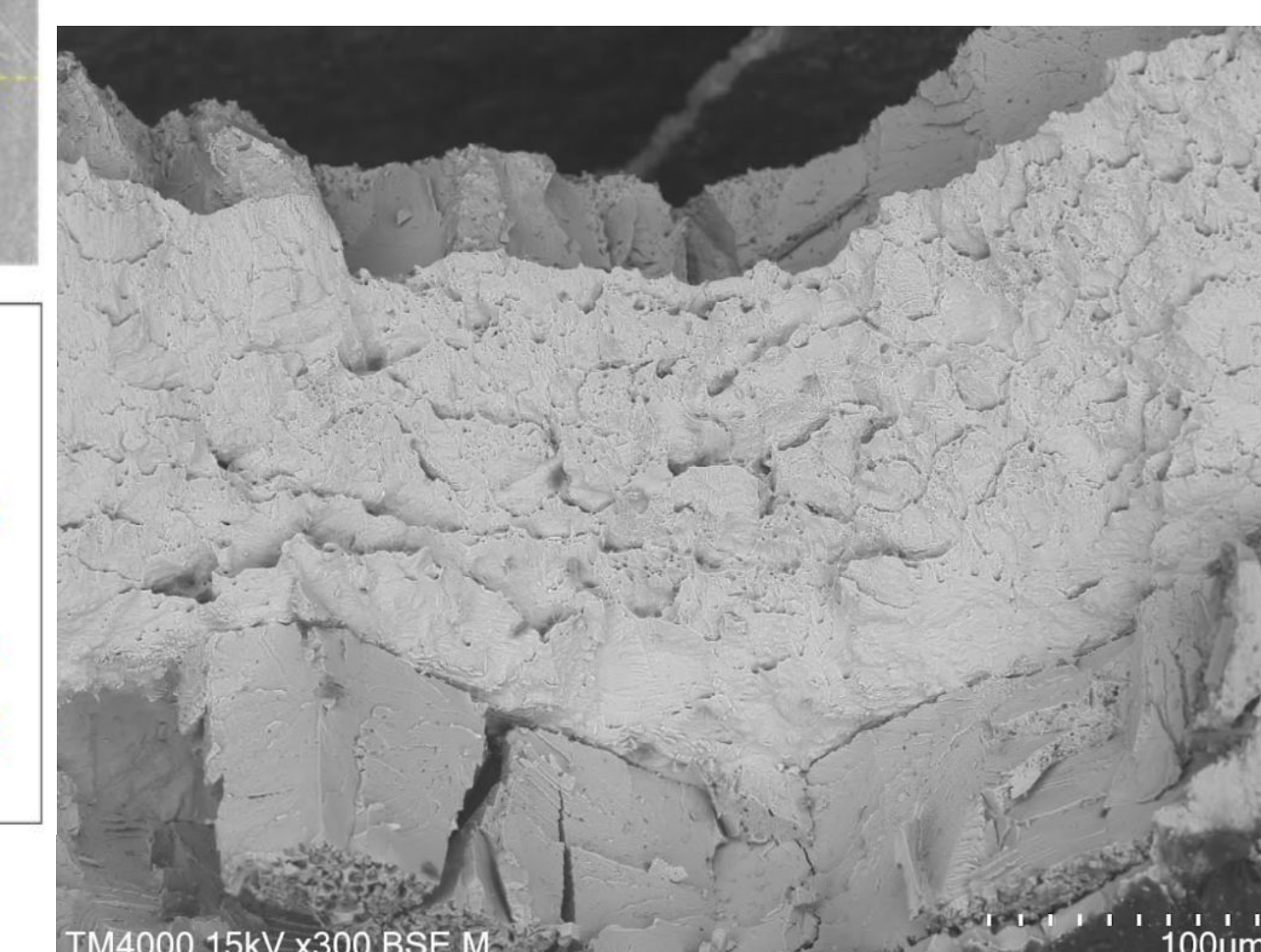
Ductile fracture of metallic layer with coherent interface shared with the first intermetallic layer visible
