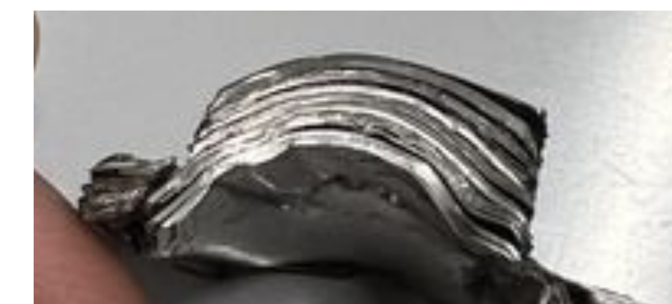
Prototype after a simulated bullet impact (sudden impact imparting ~600 J of kinetic energy)
