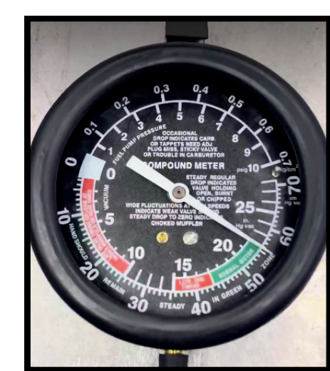
Pressure Gauge at 22" of mercury
