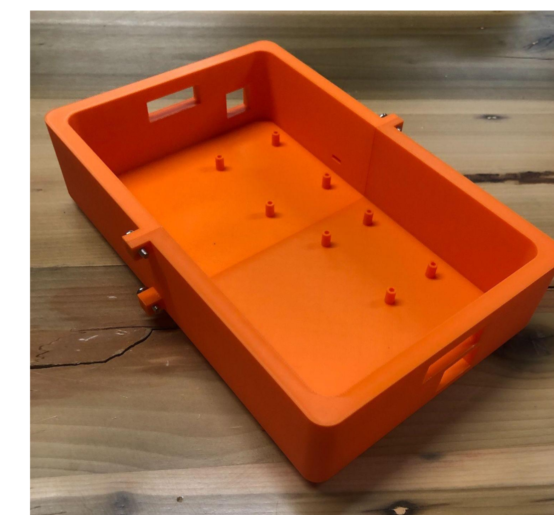
Electronics Housing Realization
