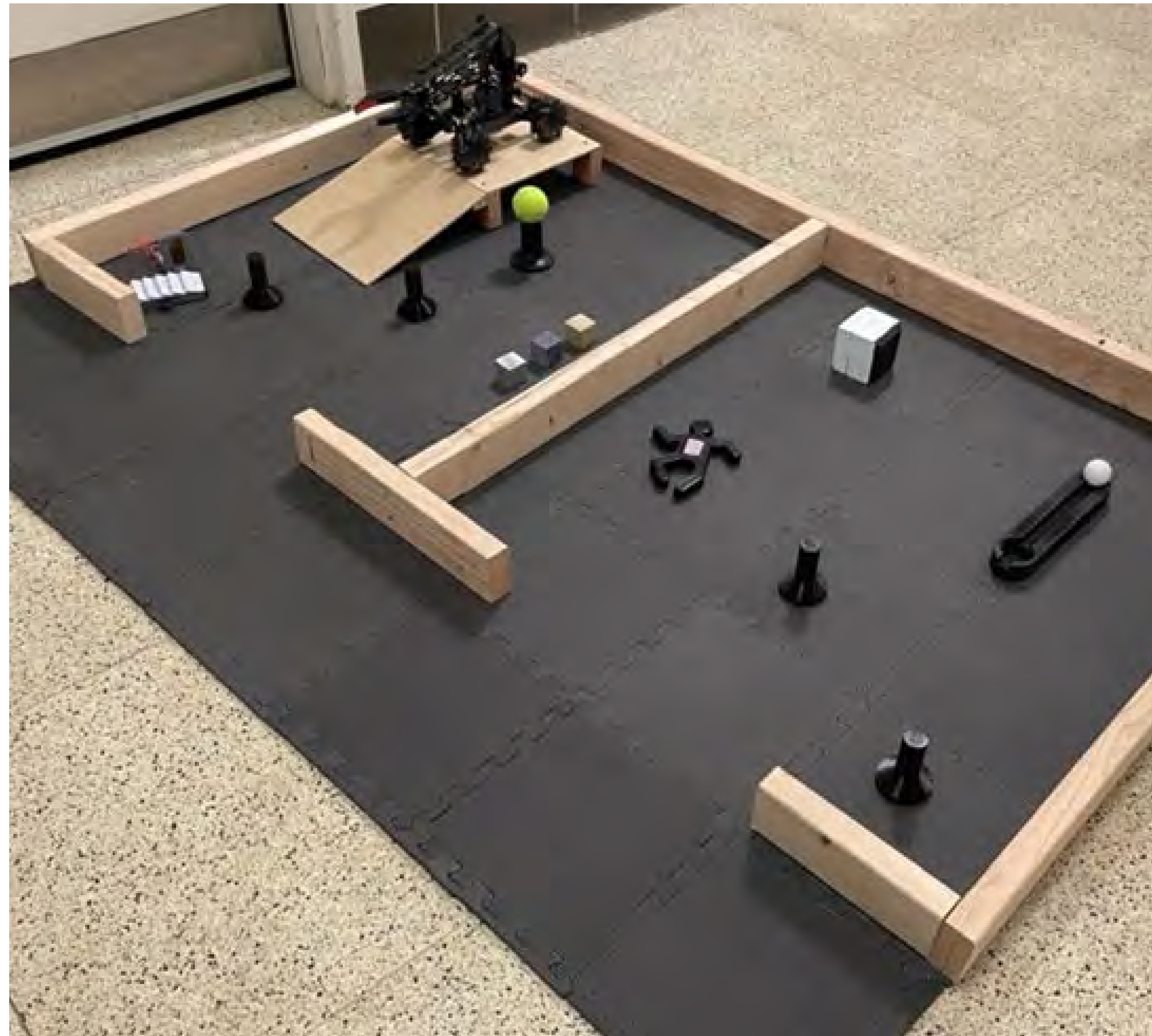
Prototypes for arena (with tasks & sample robot), detect heat task, move ping pong ball task, and 'surgery' task.
