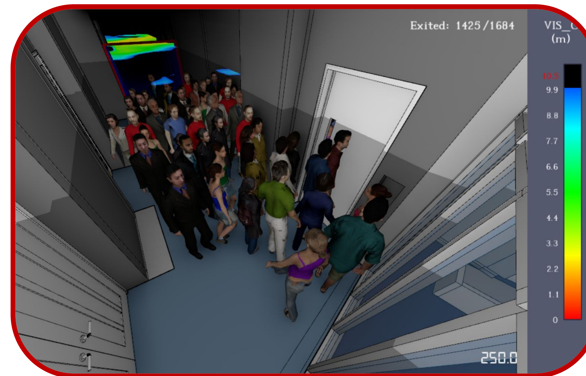
Last Occupants Egressing 2nd Floor Hallway
