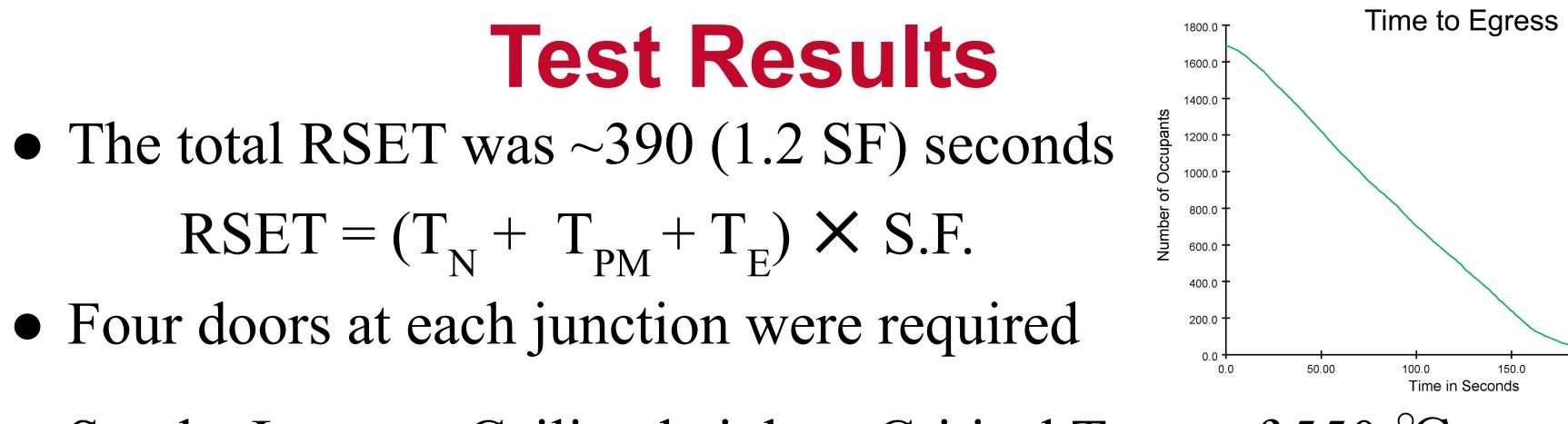
• Smoke Layer at Ceiling height < Critical Temp of 550 °C
