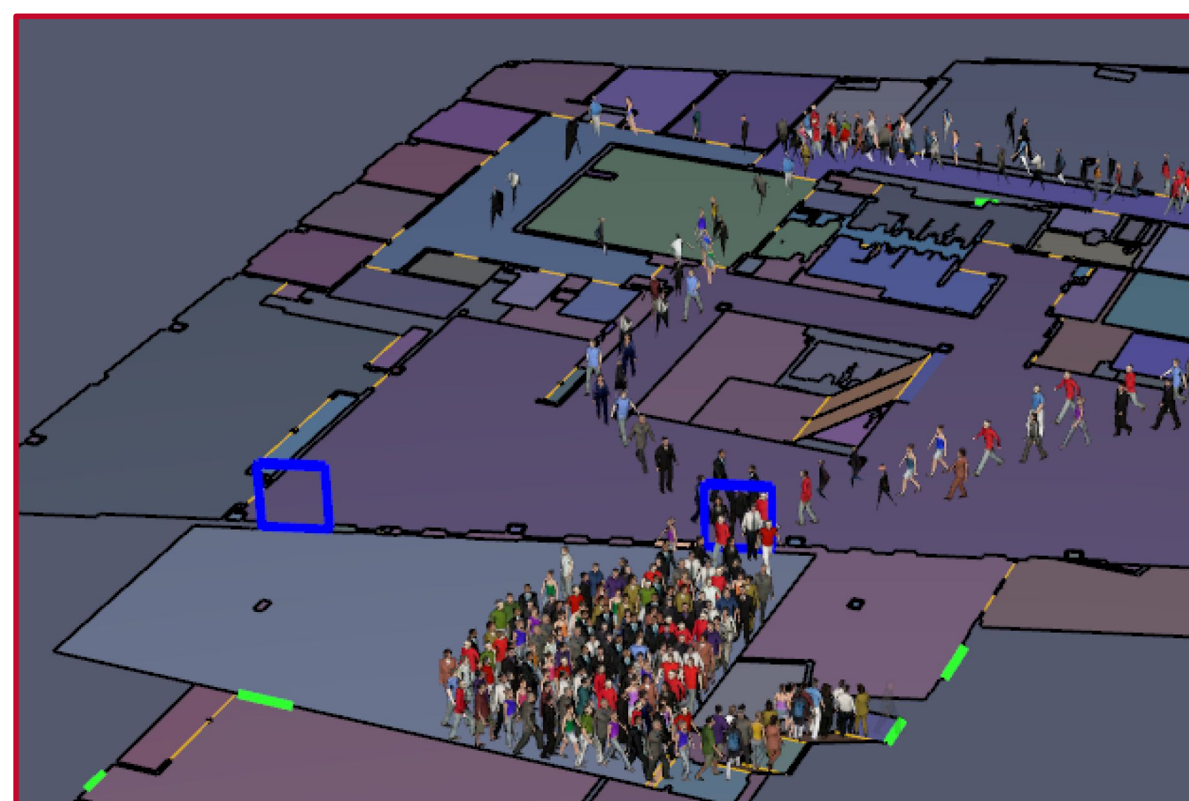
Figure 2. Second floor of pathfinder model. Queuing at the terrace shows the importance of the terrace exit. In models without the terrace stairs, egress times are higher.
