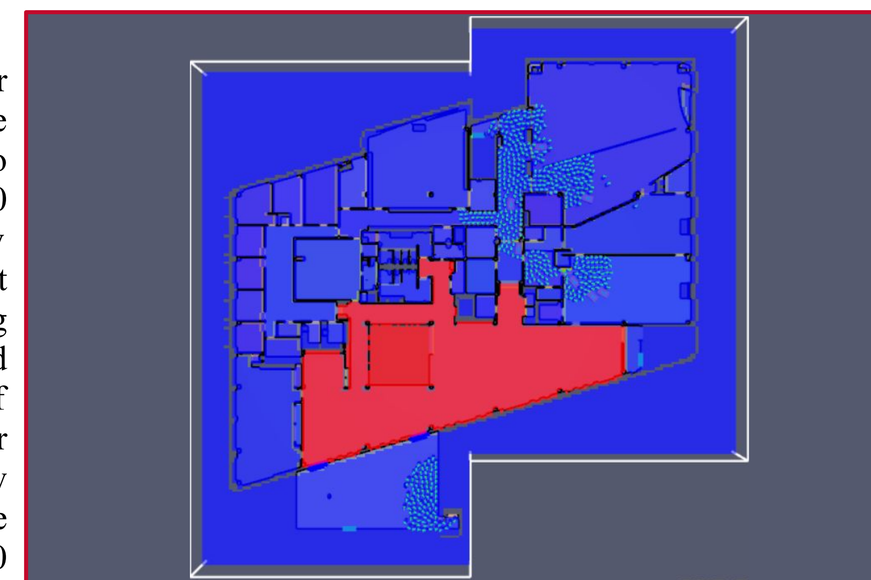
Figure 3. Visibility at 1.8 m for the second floor in the first fire scenario. Visibility less than 13 m shown in red.
