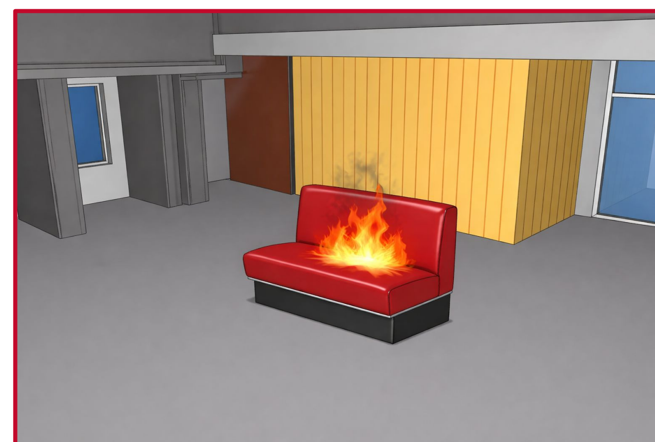
Design Fire 2: A polyurethane booth near the won-door in the cafeteria with a peak HRR of 2000 kW and a growth rate of 0.01172 kW/s 2 .
