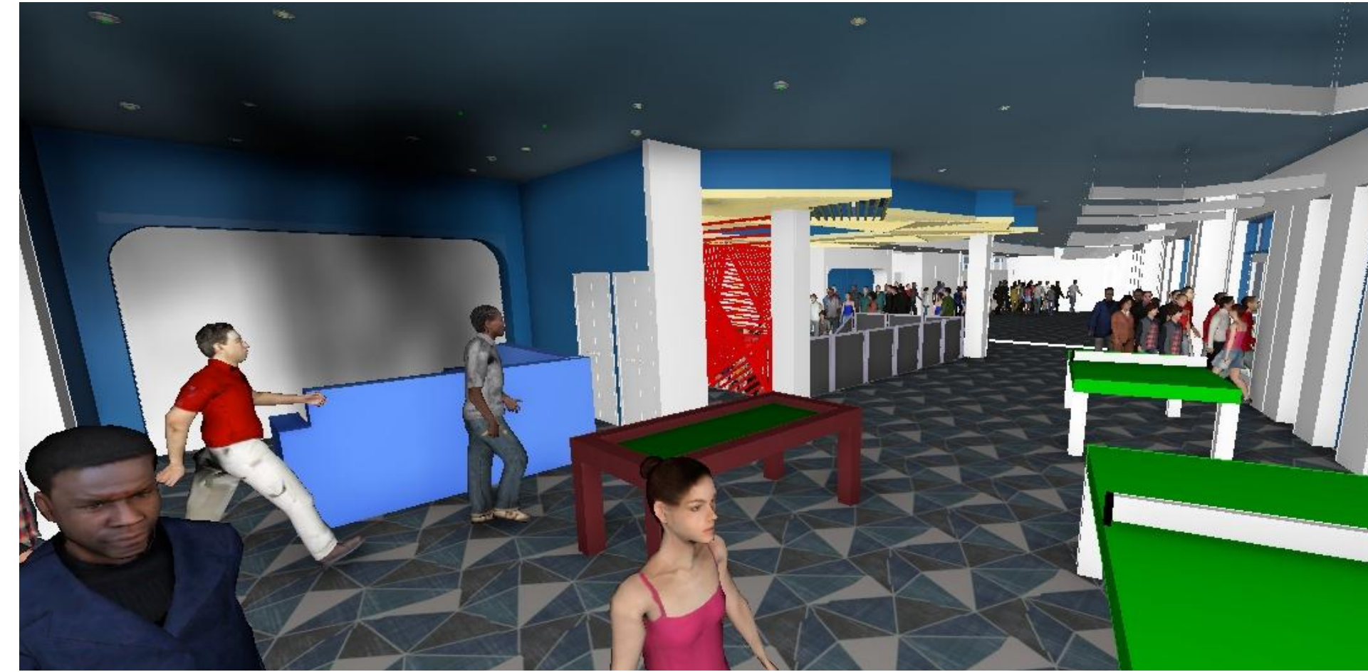
Design Fire Scenario 2: Couch fire, near the terrace exits, in the second level Student Lounge is blocked from view on three sides.
