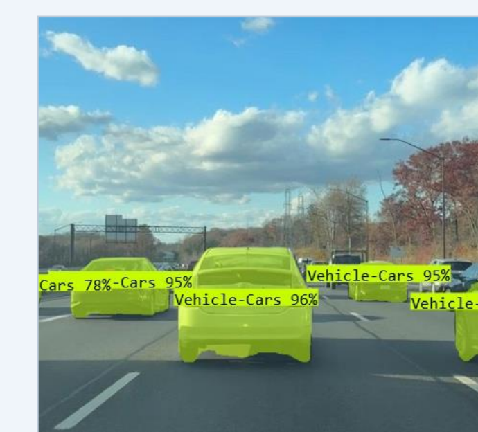
Example outputs: multi-vehicle detection with confidence overlays, and lane-departure warning when the vehicle drifts right.
