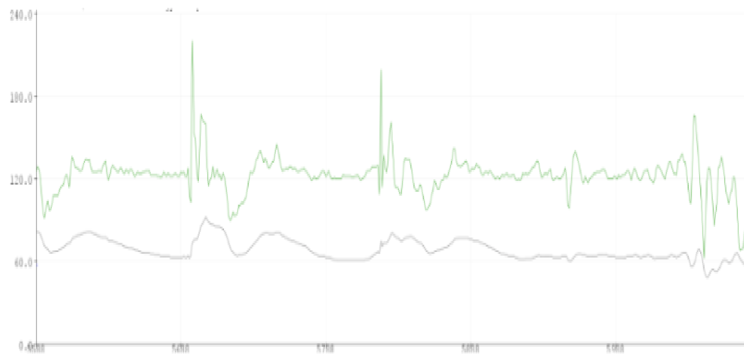
Figure 2: Acceleration data fitted with a low pass filter. Green, original signal. Black, Filtered signal
