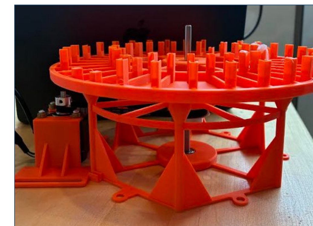
3D printed carousel, motor mount, beam break and reorientation station.
