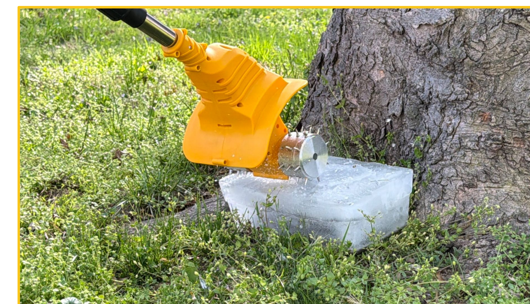
Views of prototype during testing, grinder shown (left) with testing done on ice brick (right)
