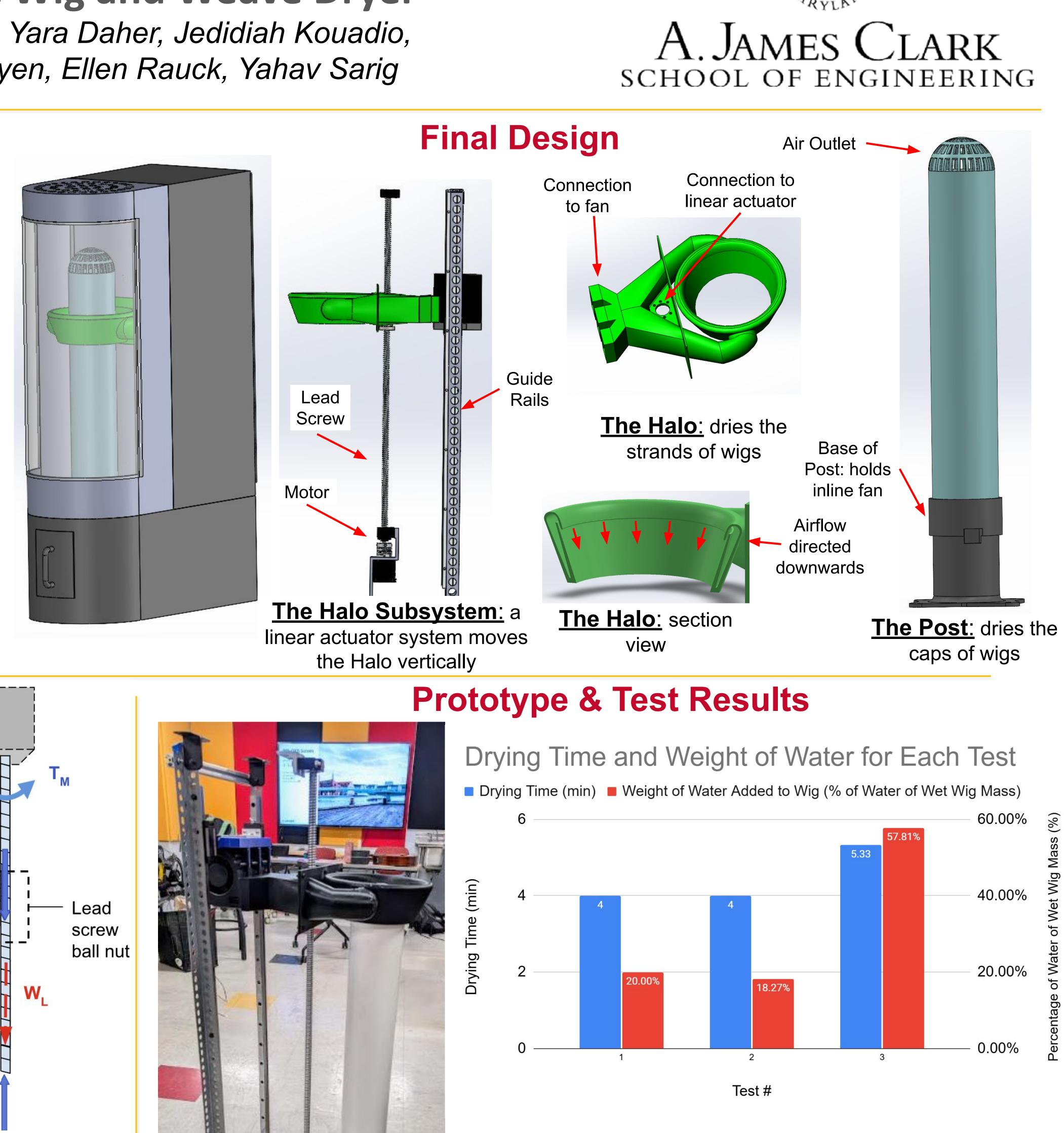
We calculated the minimum torque required for the lead screw in the linear actuator system,
