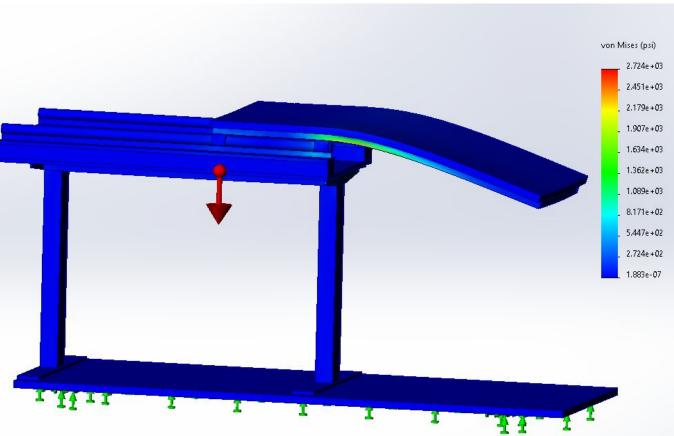
Cantilever Bending Calculation: Applied an evenly distributed 100 lb load across the top of the desk face to determine a safety factor of the design. From this experiment we determined the desk will be able to withstand a 100 lb load.
