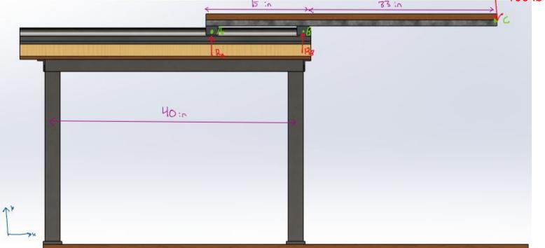
$\sum M_a = 0 = (R_b)(15 \text{ in}) - (100 \text{ lb})(48 \text{ in}) \Longrightarrow R_b = 320 \text{ lb}$  $\Sigma Fy = 0 = R_a + R_b - 100 \Longrightarrow R_a + 320 - 100 = 0 \Longrightarrow R_a = -220 \text{ lb}$
