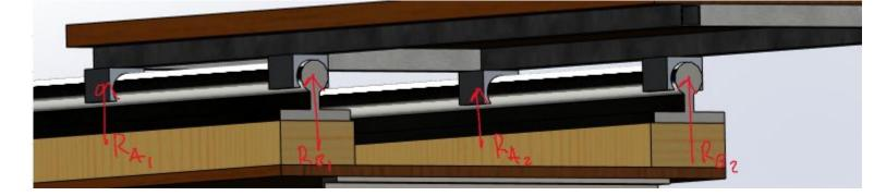
$R_{a1}, R_{a2} = -110 \text{ lb}$  $R_{h1}, R_{h2} = 160 \text{ lb}$
