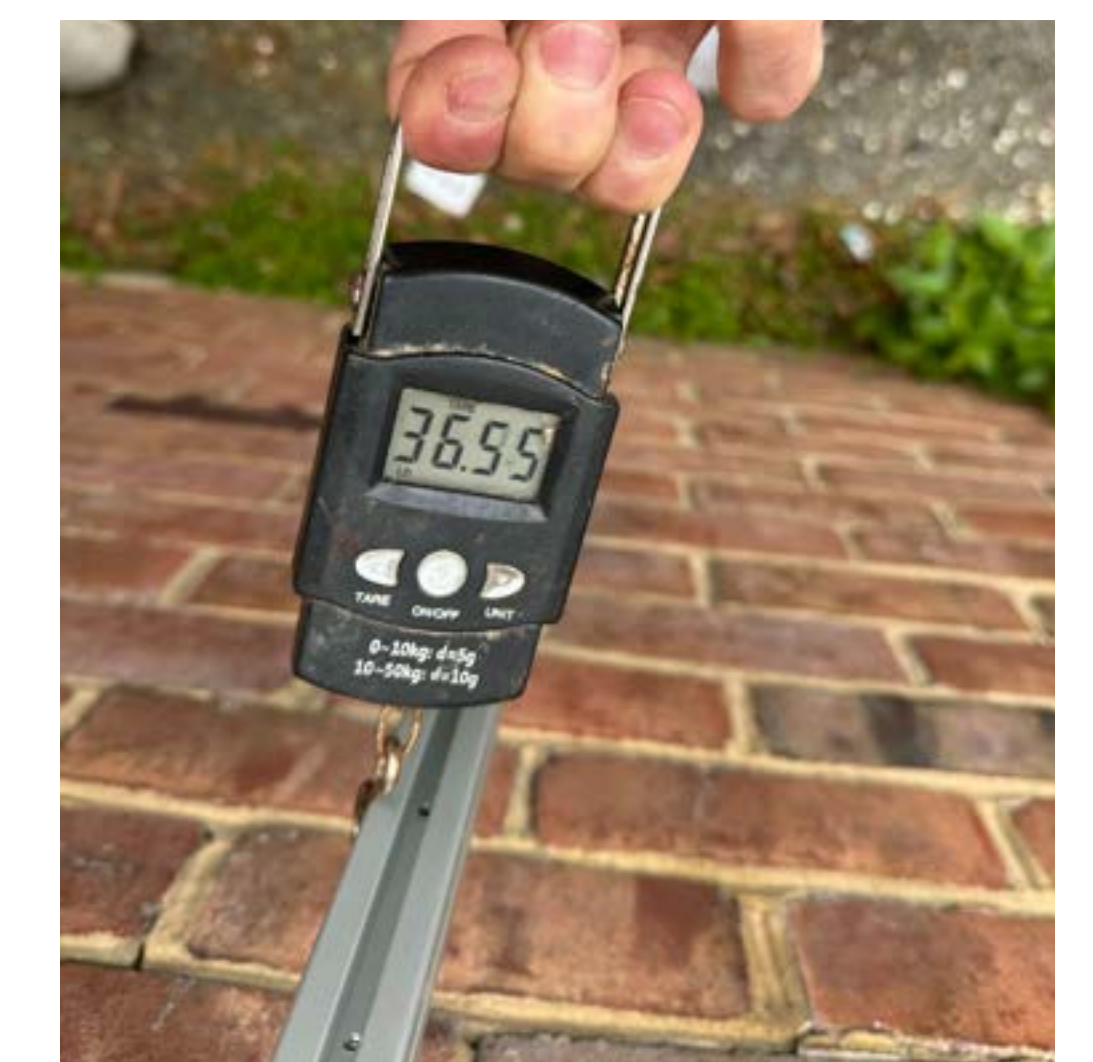
Hanging scale test to determine if sliders can withstand calculated drag forces of ~36lbf
