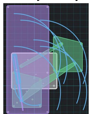
From our calculations, our linear actuator(s) should be rated for a force of at least 70.5 pounds. Stresses in linkage bars were minimal.
