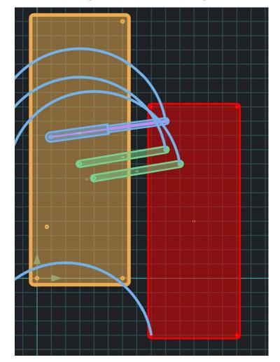
From our calculations, our linear actuator should be rated for a force of at least 237 pounds. Stresses in linkage bars were minimal.
