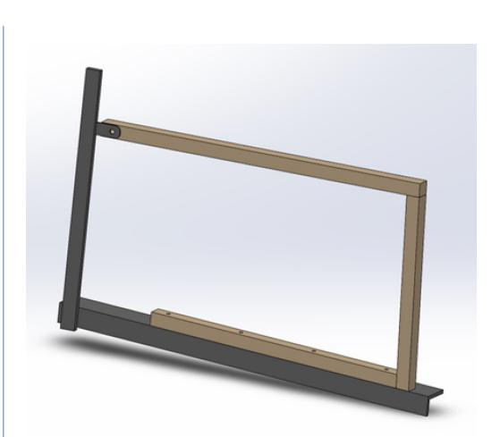
The team was also tasked with creating safer, more sturdy handrails than the existing set. The picture above shows the final setup of the handrails. These rails are bolted into the base of the treadmill and attached to the metal supports of the console for maximum sturdiness throughout.
