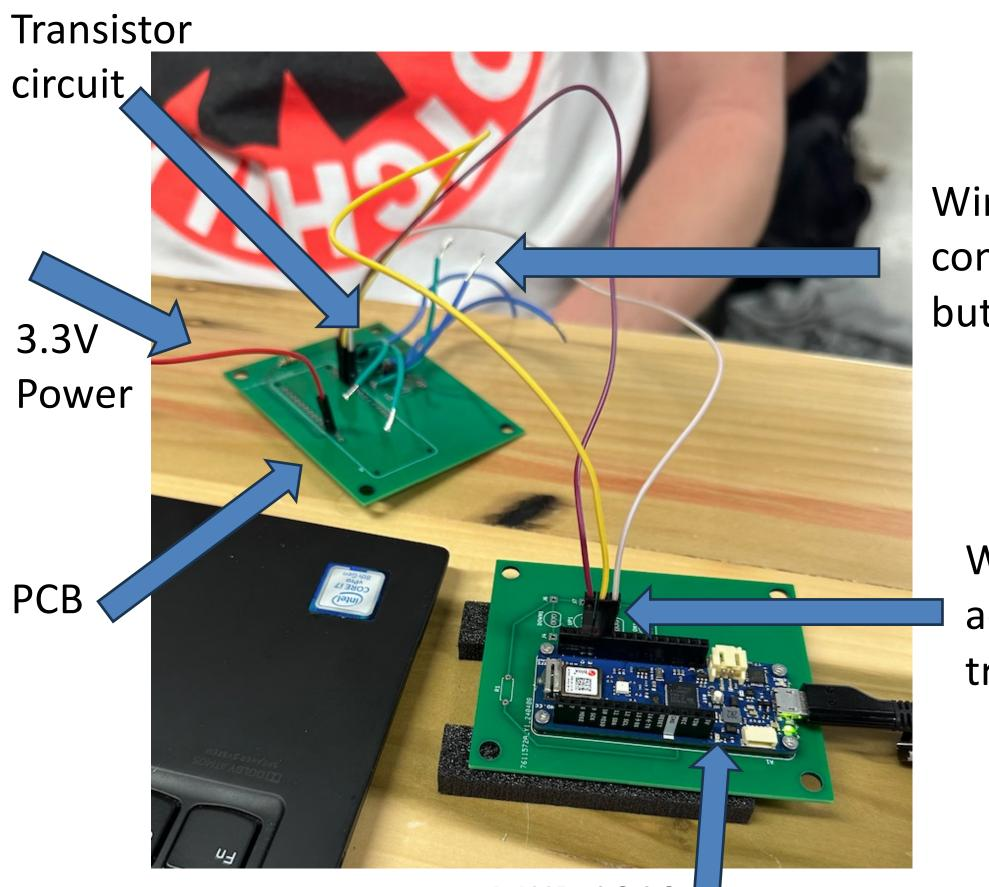
By connecting the Arduino and Alexa to the Wires to be connected to same WIFI network, the two can communicate through Arduino IDE and the Alexa app. This button leads will allow the commands spoke by the user to be understood by the Arduino's setup.
