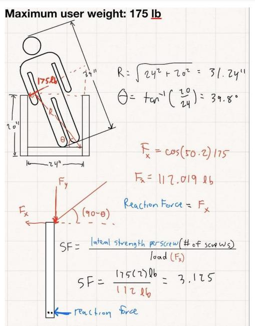
Simulated Finite Element Analysis (FEA), was not conducted due to the inconsistent isotropic properties of wood. Instead, hand analysis of the wooden handrail joint was considered.
