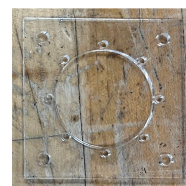
Acrylic laser-cut plate as valve building foundation
