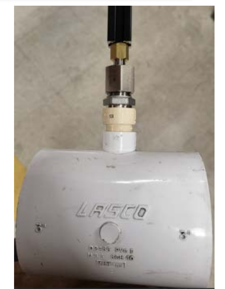
First iteration of waterproof enclosure and rail connection
