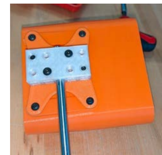
First iteration of connection between sonar and rotating shaft
