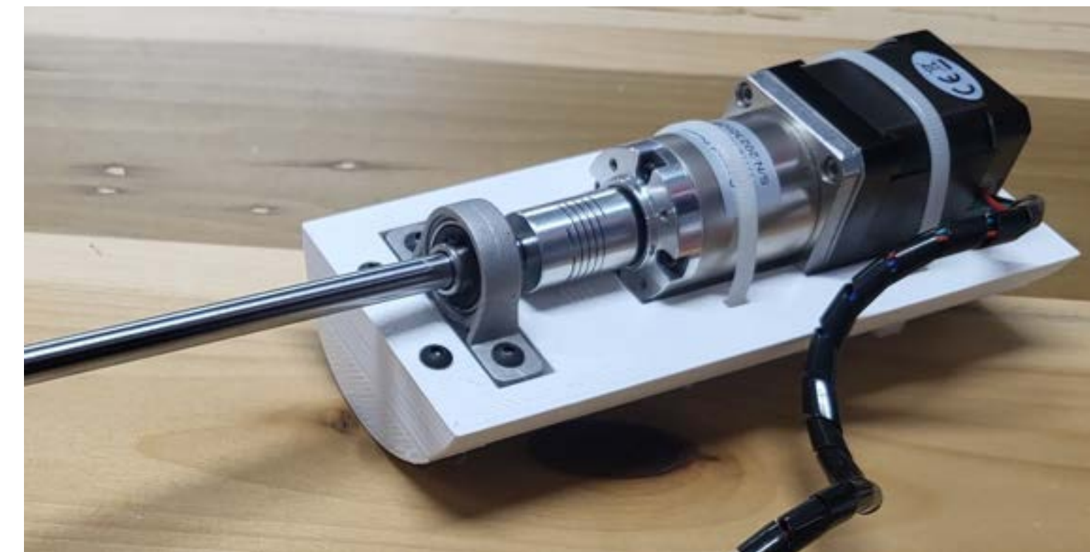
Assembly inside the waterproof enclosure that provides angular actuation
