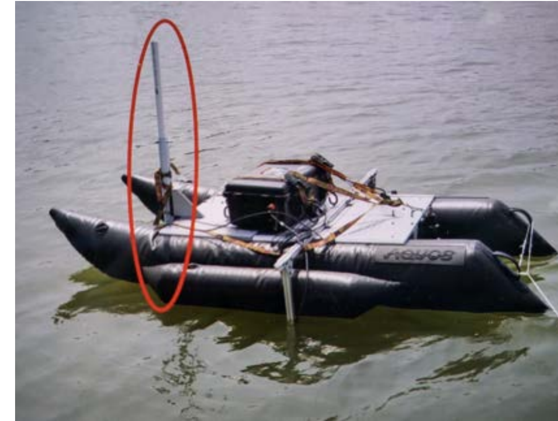
Current Autonomous Surface Vehicle (ASV) set-up with manual depth adjustment.
