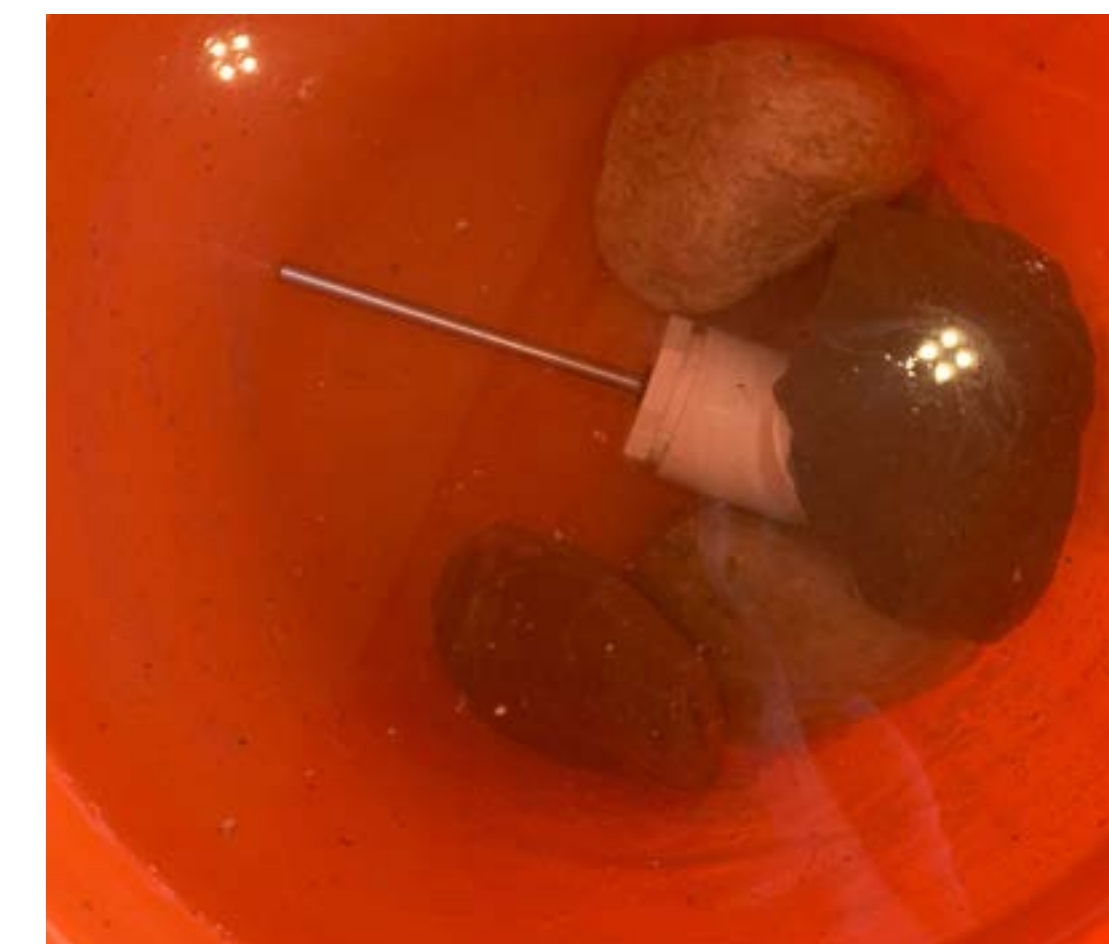
Waterproof Assembly submerged under water (rocks use to hold assembly down)
