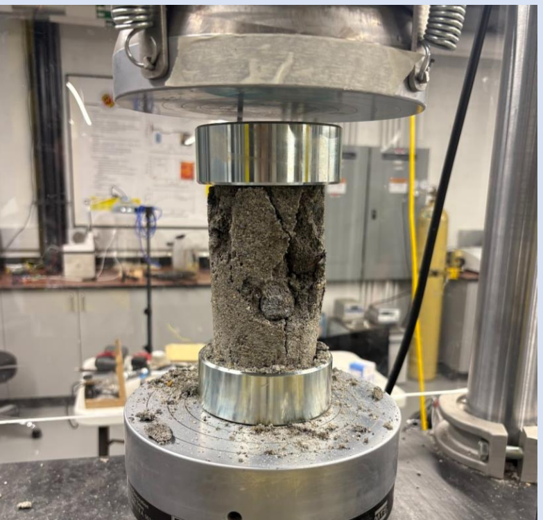
30% Biochar Compression Testing Failure
